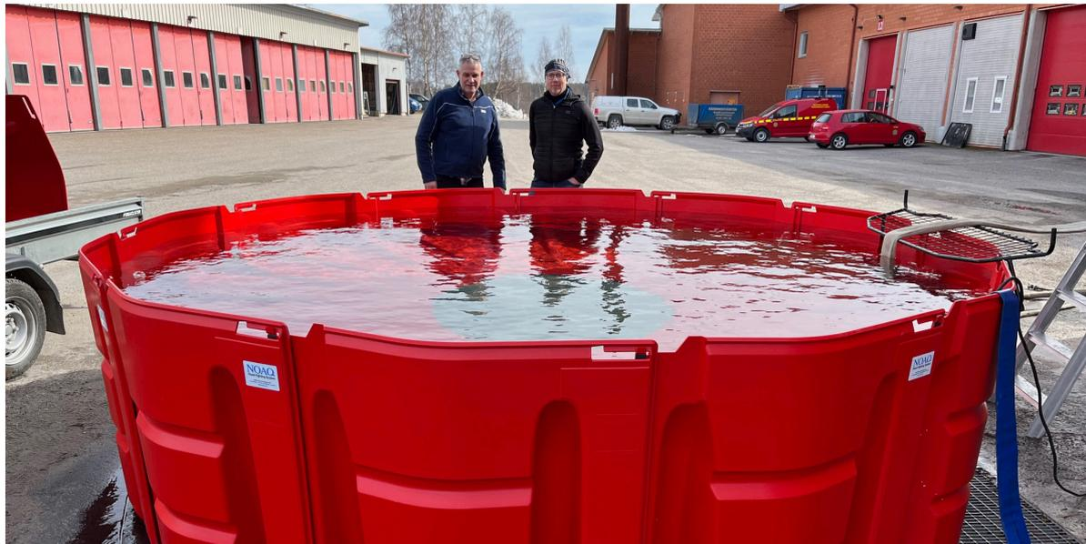
*"It is always really interesting and fun to see how such a light construction as a Boxwall can withstand the water pressure"- says Conny Löftstedt, product designer at NOAQ. Each of the 12 corner boxes weighs no more than 13 kilos, but in this Boxpool configuration they can hold in place no less than 9 tons of water.*
